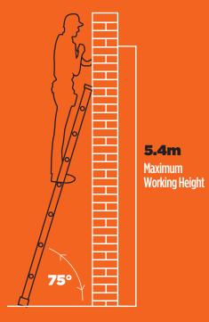
Max Working height is calculated as Max Standing height + 1.6m
