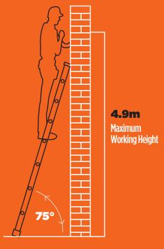
Max Working height is calculated as Max Standing height + 1.6m
