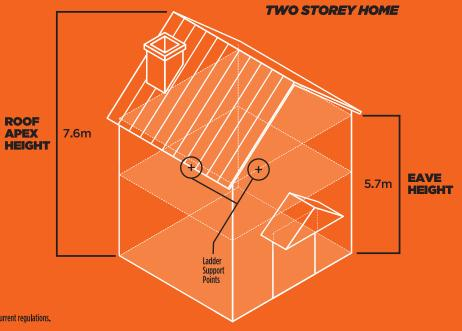
All dimensions in metres. All measurements are typical of UK homes built to current regulations.
